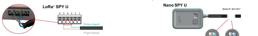
RACCORDEMENT SUR CONTACT SEC / DRY CONTACT WIRING
