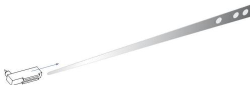
Remove the point protector by pulling and turning it simultaneously.
